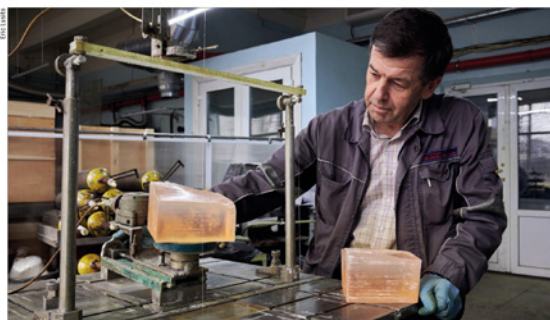
Photo 8 A technician processing alkali-halide scintillation crystals at the Institute for Scintillation Materials, Kharkiv.
